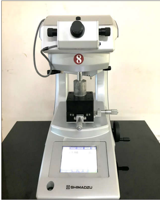
Fig. 2. Specimen loaded on (Shimadzu) hardness tester
